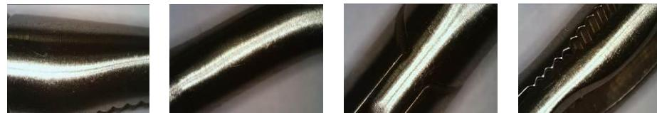
Because the tongs are made of metal material, the reflection of light is inevitable due to the low surface roughness.
