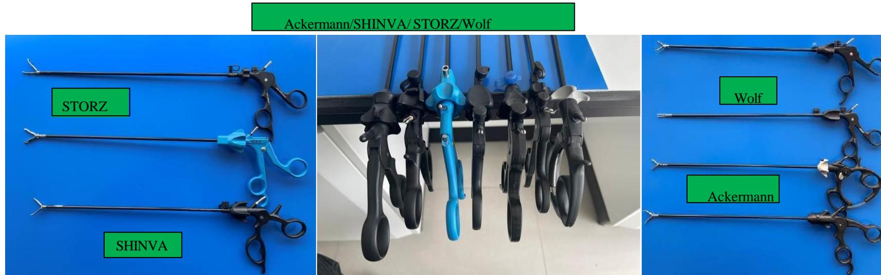
There are no burrs or other defects that may cause injury on the external surface of the products of the four brands. Overall structure, Wolf brand and Ackermann products have no flushing interface components.
