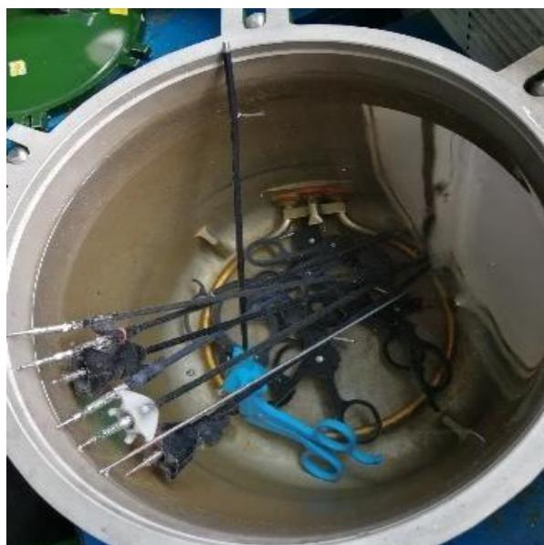
**There is no surface corrosion, crack and other defects in the above four grasping pliers, indicating that the materials of each Brand and SHINVA grasping pliers are properly selected, and after sterilization according to the standard requirements, there will be no rust and micro cracks in the grasping pliers after operation.**
