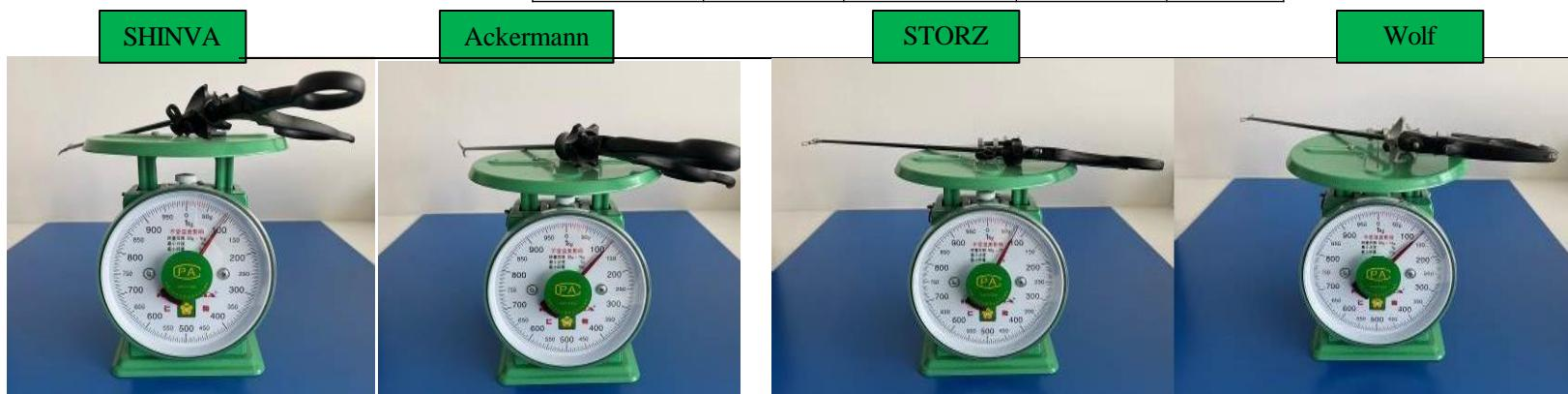
Ackermann and Wolf products weigh 18-47g heavier than other brands due to their wide handle structure design. STORZ products because of its runner and handle design are relatively small, according to the characteristics of Chinese people have been specially designed, the weight is as low as 78g, long time use is more labor-saving; **SHINVA weighs 94 grams, which has some advantages over other products.**
